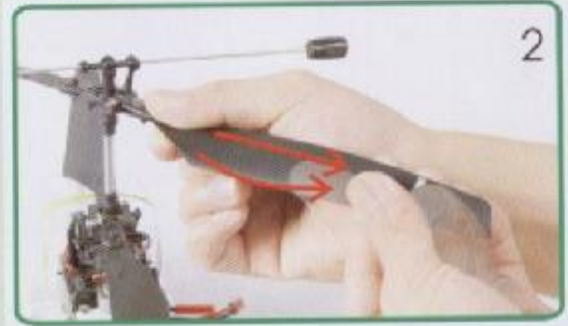
(2)主旋翼攻角调整方法 Adjustment way to angle of attack of main blades.
