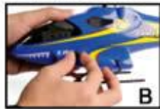
拔下前纽扣，取下前机头罩 Pull out the front fastener and take the front canopy.
