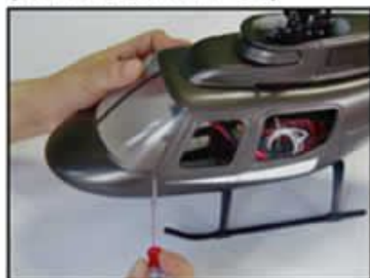
把座仓装上 (自攻螺丝: 1.4*5mm 4个) Assemble the cabin. (Self-tapping screw: 1.4*5mm 4PCS)
