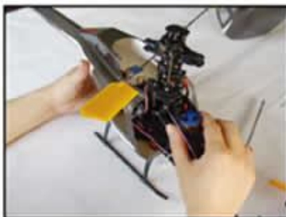
将主机架放进机壳 Put the main body into the scale cabin.
