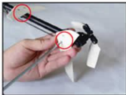
将平尾，垂尾，滑撬拆下。 Disassemble the tail paddle, and vertical fin and landing skit.
