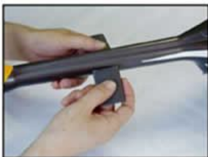
用AB胶把平衡尾粘好 Stick up the tail paddle with AB glue.
