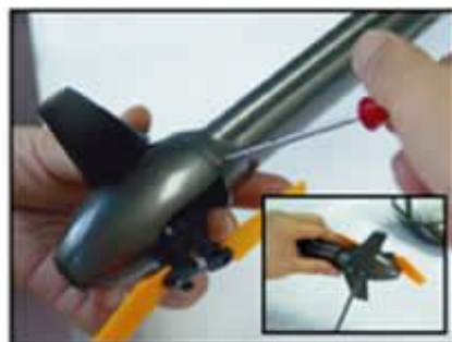
把尾罩用螺丝固定好 (自攻螺丝: 1.4*5mm 3个) Fix the tail cover with screws. (Self-tapping screw: 1.4*5mm 3PCS)
