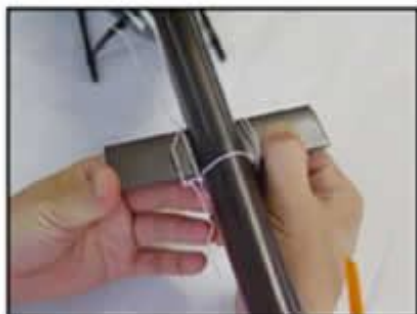
把接收机天线绑在平尾上 Tie up the receiver antenna on the tail paddle.
