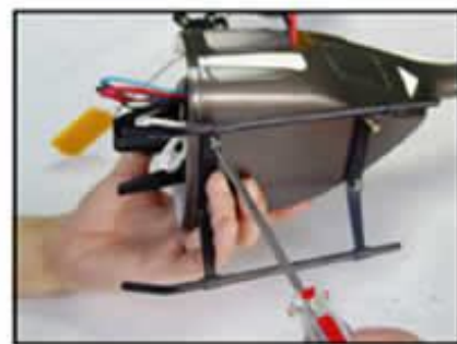
用螺丝把滑撬与主机架固定好 (螺丝: 2*25mm 4个) Fix the landing skit and the main frame with the screws. (Screw: 2*25mm 4PCS)
