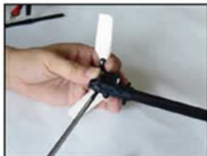
将尾箱拆下，拉杆取下。 Disassemble the tail box and remove the push-rod.
