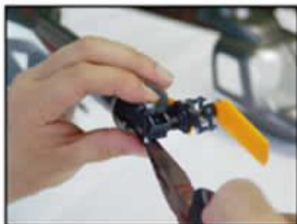
将尾箱装上并套上拉杆 Assemble the tail box and fit on the push-rod.
