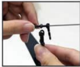
A Stabilizer set disassembling
