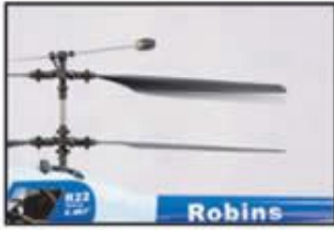
Main blades don't rotate in one plane 主旋翼旋转不在同一平面
