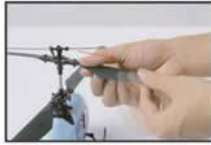
Adjustment way to angle of attack of main blades 主旋翼功角调整方法
