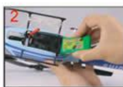
2 Loading battery 安装电池
