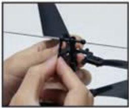
A Stabilizer set disassembling
